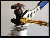
SLOWLY turn the valve on top of the tank. The hose may move as the liquid CO2 enters the hose and makes it stiff. Check for any leaks you may see as you open the valve more. If you notice leaks, turn off the valve and locate leaks. Once located contact CryoFX. When finished using, turn valve on top of tank in opposite direction as the last time you turned it so as to close the valve. Activate Cryo Jet a few more times to let the remaining CO2 in the hose out.
