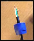
Slide the white piece onto the wires as shown. Connect the wires to the terminals as shown below; Black - L (Live), Green - (Ground Symbol), White - N (Neutral). Slide the white piece forward.
