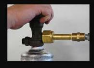
WARNING: Co2 Blasts cannot exceed 3 seconds in length for each blast. Two blasts cannot occur within 5 seconds of eachother. Power must be connected last as to ensure safety.
