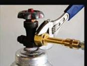
4. SLOWLY turn the valve on top of the tank. The hose may move as the liquid CO2 enters the hose and makes it stiff. Check for any leaks you may see as you open the valve more. If you notice leaks, turn off the valve and locate leaks. Once located contact CryoFX. When finished using, turn valve on top of tank in opposite direction as the last time you turned it so as to close the valve. Activate Cryo Jet a few more times to let the remaining CO2 in the hose out.
