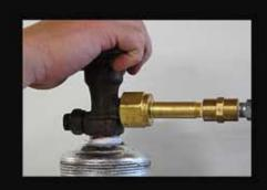
4. Grab the Cryo-Gun and slowly squeeze inner handle to spray CO2. Make sure you have a firm grip as the Cryo-Gun may slip out of your hand while spraying. When finished using, turn valve on top of tank in opposite direction as the last time you turned it so as to close the valve. Return to Cryo-Gun and squeeze handle to let the remaining CO2 in the hose out.
