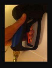
WARNING: NEVER disconnect the Cryo-Gun from the hose or unscrew the hose from the Co2 tank while there is pressure in the hose. Turn off valve and squeeze handle to release pressure beforehand
