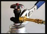
3. SLOWLY turn the valve on top of the tank. The hose may move as the liquid CO2 enters the hose and makes it stiff. Check for any leaks you may see as you open the valve more. If you notice leaks, turn off the valve.
